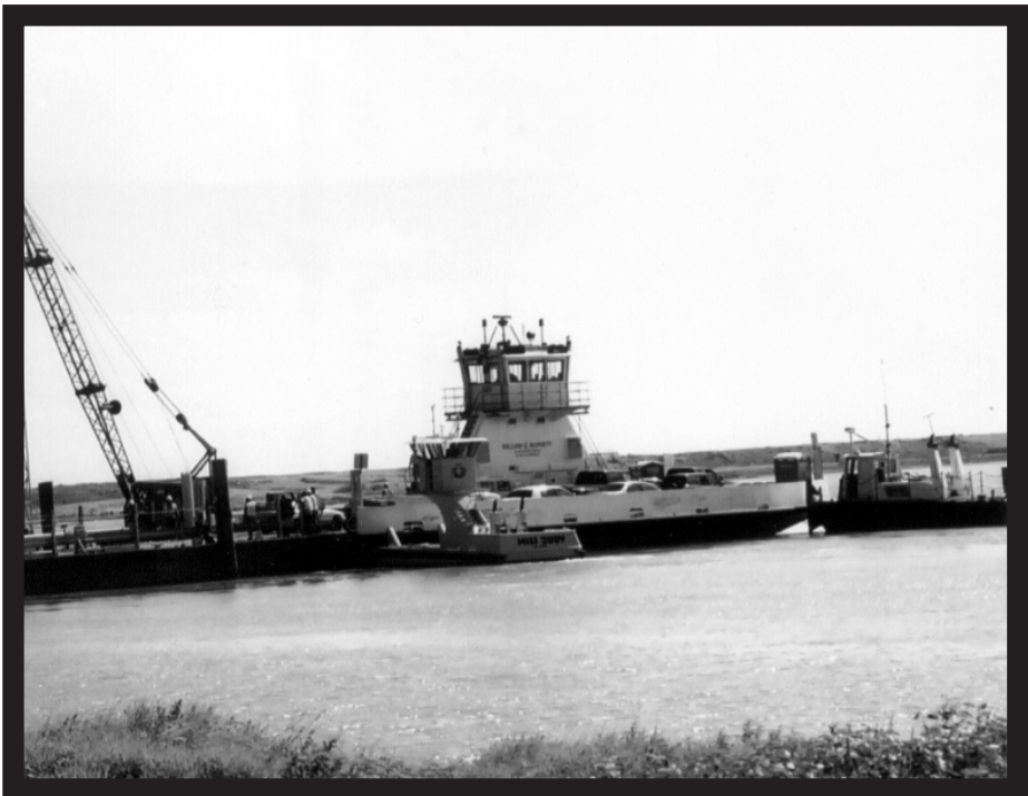
Mating the car ferry with the barge, it only took two harbor tugs. a
